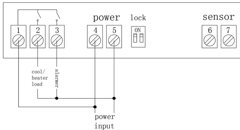
Terminals 1 and 2: Connect the cooler or heater
