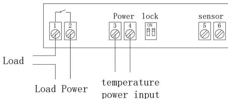
Terminals 1 and 2: The output of cooling and heating.
