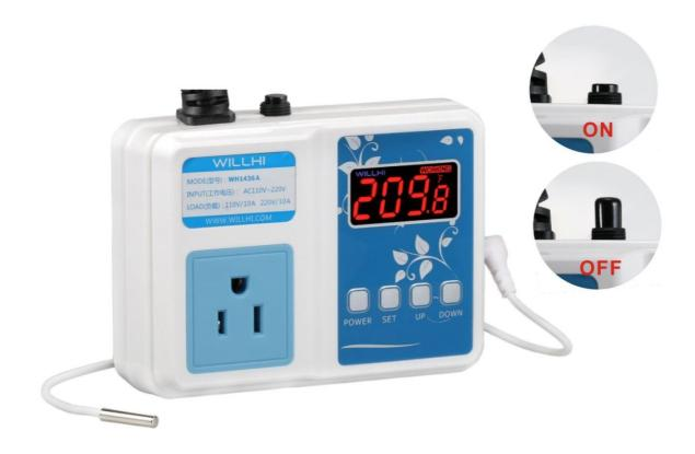
Wew Safety Feature: The fuse reset button pops out when a short or overloading is detected. If the fuse reset pops out, the short or overloading condition must be fixed before the button will stay pushed in. Do not manually hold the button in as this will create a dangerous condition. The button needs at least 2cm(0. 8 inches) clearance to pop out. Be sure it's not blocked.
